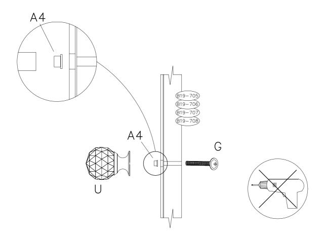
CAUTION: Please ensure that the spacer A4 is in position before you fixed the handle to the drawer front. Only hand tighten the handle, overtightening or missing the spacer could damage the mirrored drawer fronts.
